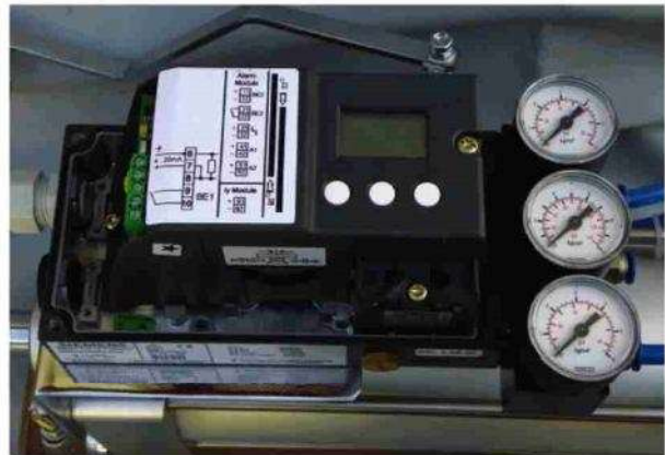
Electro-Pneumatic Cylinder with Type Electro pneumatic Positioner
