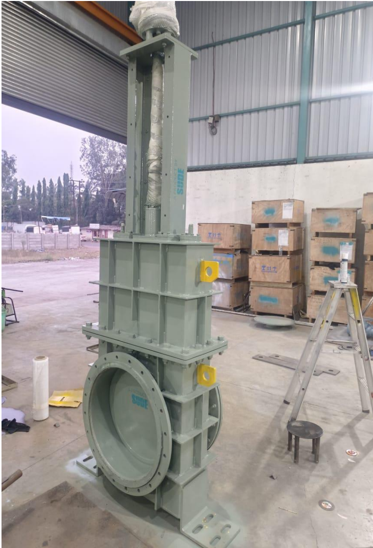
FINISHED VALVE AFTER FINAL PAINTING
